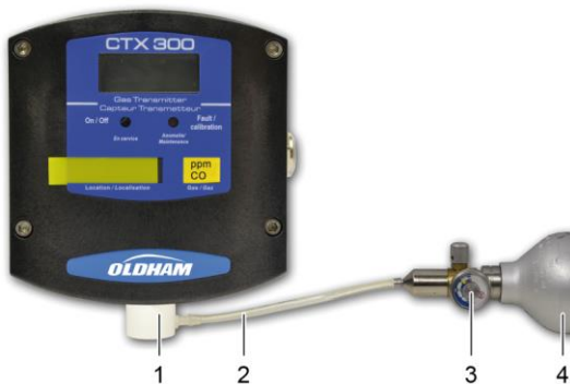
Figure 14: sensor calibration assembly.
