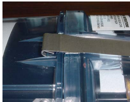
Fig. B. Incorrect band position
