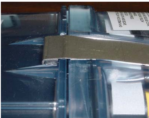
Fig. A. Correct band position.
