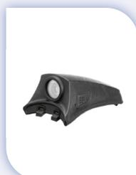
The particularly light LED helmet lamp illuminates your entire work area. It has effective anti-glare protection. The high power LED has three modes (bright, dim, off). The battery charge level is displayed during use. IECEx: Ex ib IIC T4 / T3 Gb, ATEX: II 2G Ex ib IIC T4 / T3 Gb
